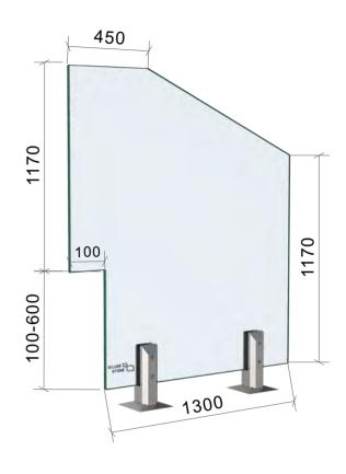
Drawing ID C1170 Drawing ID C1170T Drawing ID C1170TC
